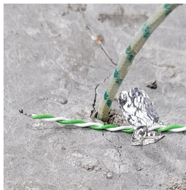
Figure 12: Thermocouples installed inside and on the surface of the concrete specimen to monitor the temperature during thermal heating.
