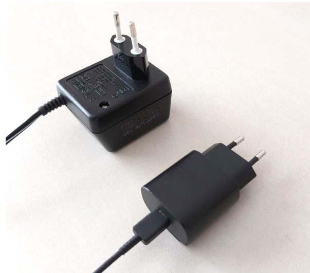
Fig. 2.19. Illustrative comparison between a 50 Hz transformer-rectifier (top left) and a solid-state transformer (bottom right)
