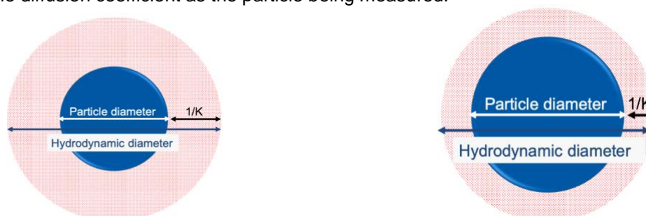
Figure 2.14 shows the particle diameter, hydrodynamic diameter and its thickness (Figure source, A.P Instrument)
