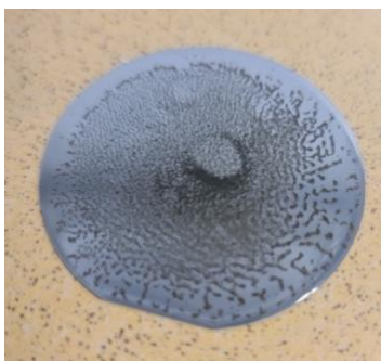
Figure 3.9 showing sample of nanodiamond droplet on silicon glass surface
