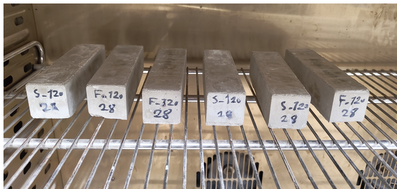
Figure 3: The prism specimens located inside the heating chamber for thermal activation [42].
