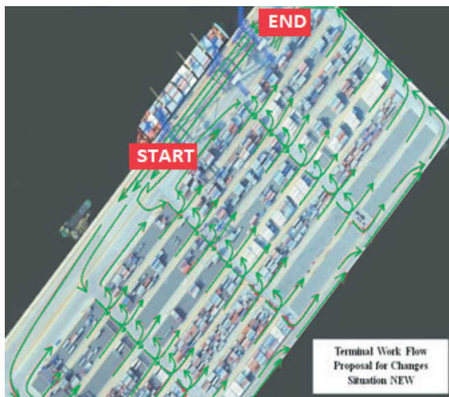
Fig. 10. Terminal workflow after rotating the containers in the yard
