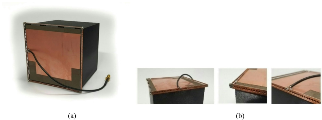
Fig. 14. Fabricated CubeSat antenna: (a) perspective view, (b) diverse side views.
