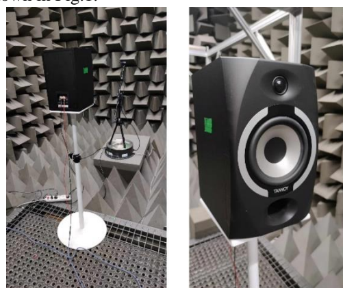
Fig. 1. Directivity measurement setup
