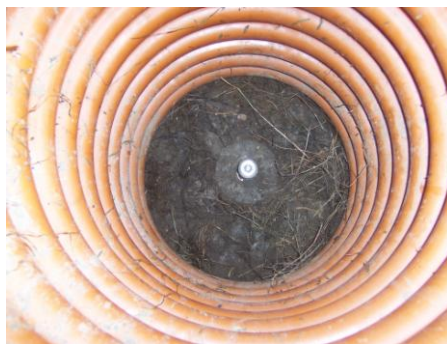
Fig. 6. A view of a benchmark at a check point.
