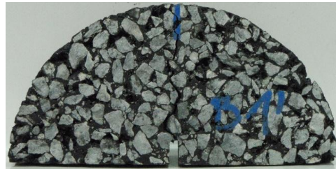
FIGURE 2. Stone matrix asphalt PA 8.
