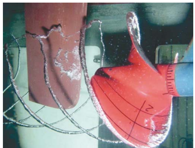
Fig. 1. Cavitating tip vortices shed from the blades of the marine propeller model and interacting with the ship rudder (courtesy of the Ship Design and Research Centre CTO S.A. in Gdansk, Poland)
