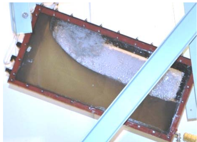
Figure 2. Exemplary shape of a free surface of liquid inside a partly filled model tank (own research) – it may be clearly seen that the free surface is far different than assumed within the quasi-static approach (ref. to Fig. 1)
