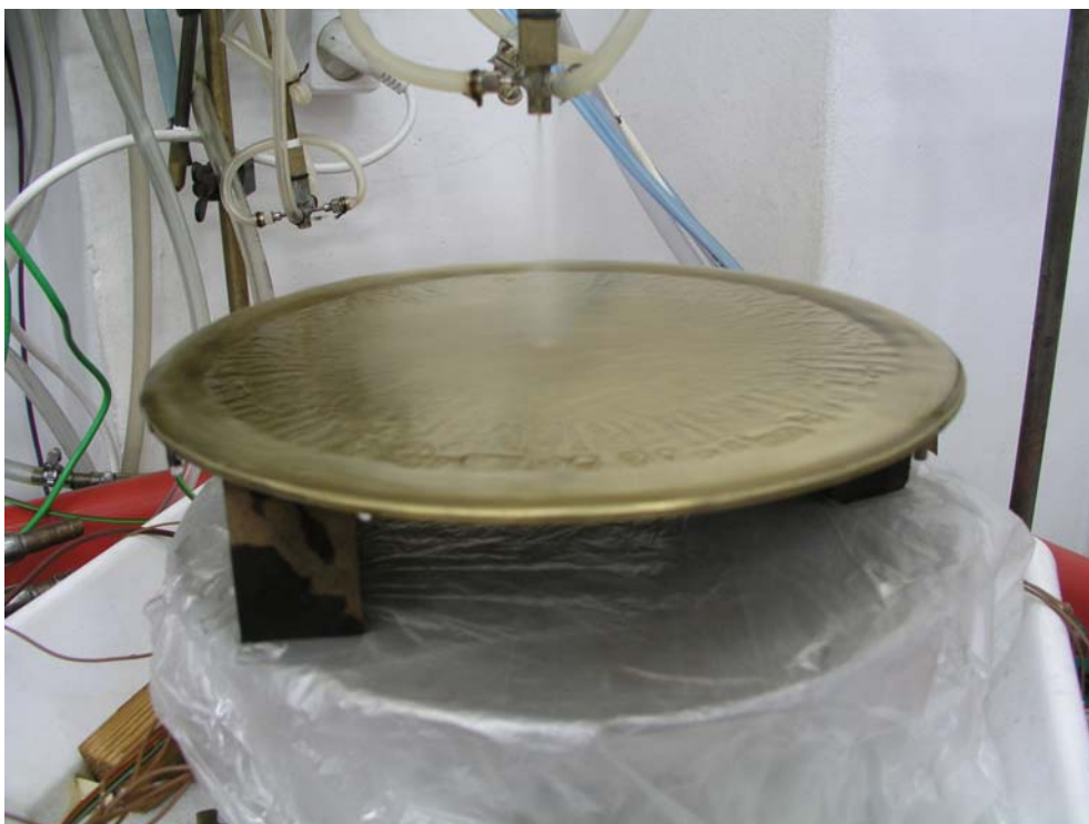
Fig. 12. Phenomenon of re-wetting of liquid layer on a brass surface, following the increase of liquid flow rate from the parameters in Fig. 11 to Re_g=89\ 894 , Re_l=1971 .
