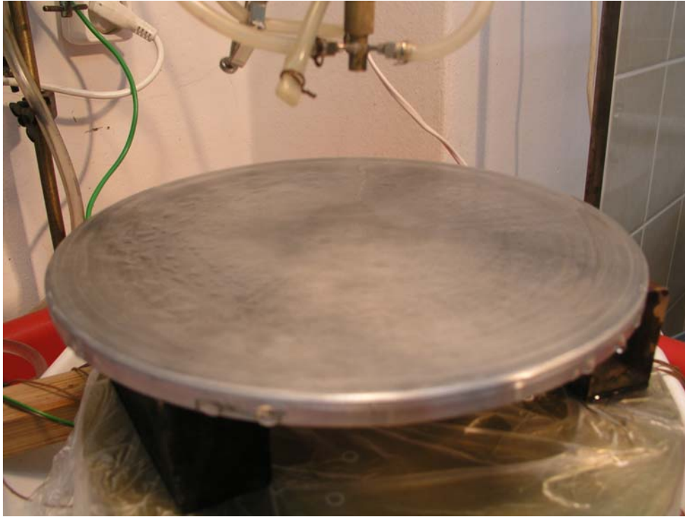
Fig. 13. Phenomenon of breakdown of continuous liquid layer on a aluminum surface, view after the breakdown, Re_g=81\ 336 , Re_l=555 .
