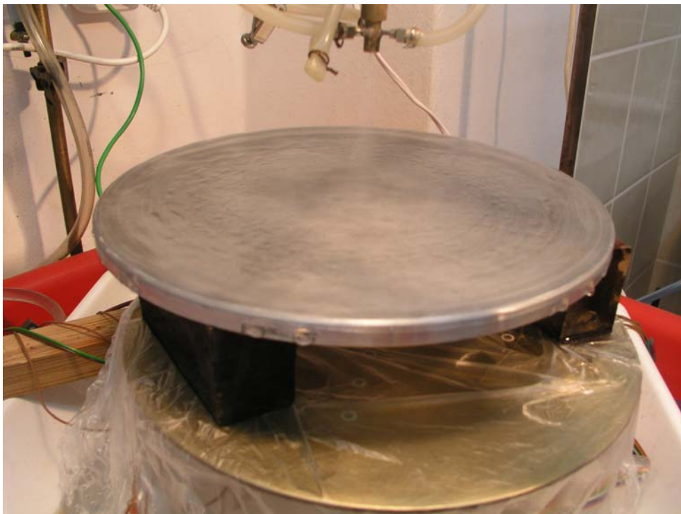
Fig. 14. Phenomenon of re-wetting of liquid layer on a brass surface, following the increase of liquid flow rate from the parameters in Fig. 13 to Re_g=81\ 558 , Re_l=1171 .
