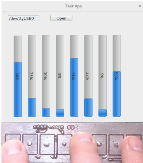
Fig. 14. Multitouch sequence and observed signals - three fingers touch
