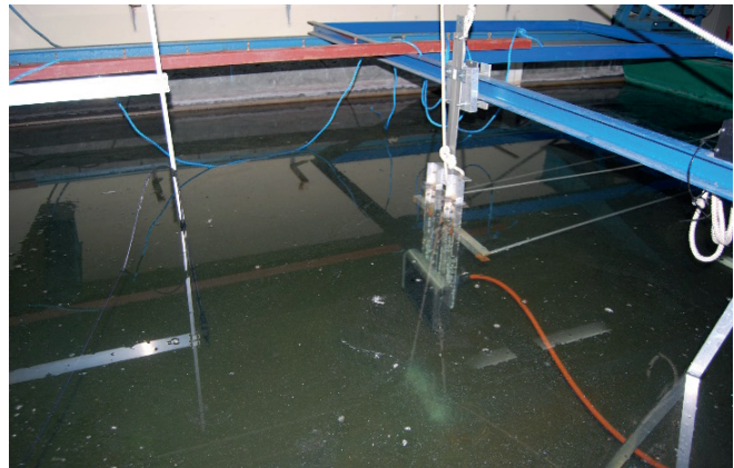
Fig. 6. Parametric echosounder antenna on support
