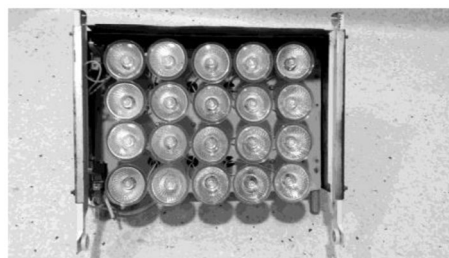
Figure 5. The 1000 W matrix of halogen lamps used in the research as heating excitation.
