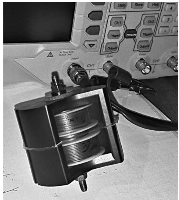
Fig. 7 Transformer used in experimental tests
