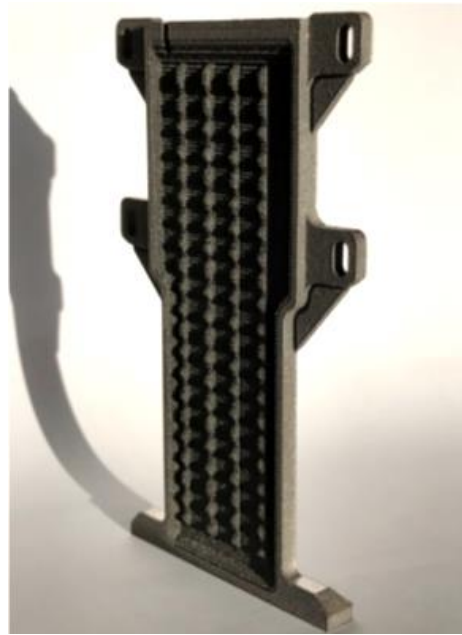
Figure 15. Titanium AM vapour chamber HP with integrated lattice structure [17].
