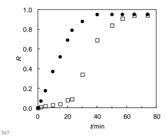
**Fig. 5.** Changes of the Al (●) and Cu (□) removal ratio with the flotation time:  $c_{0\text{Al}} = c_{0\text{Cu}} = 1.5 \times 10^{-4} \text{ mol dm}^{-3}$ ,  $u_{\text{G}} = 1.51 \times 10^{-3} \text{ m s}^{-1}$ ,  $c_{\text{SDS}} = 0.940 \times 10^{-3} \text{ mol dm}^{-3}$ , pH = 3.0.
