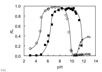
Fig. 1. Influence of the initial pH on the Al  $(\circ, \times)$  and Cu  $(\blacksquare, +)$  final removal ratio using SDS  $(\circ, \blacksquare)$  and CTAB  $(\times, +)$ .  $c_{0\text{Al}} = c_{0\text{Cu}} = 1.5 \times 10^{-4} \text{ mol dm}^{-3}$ ,  $c_{\text{SDS}} = 1.25 \times 10^{-4} \text{ mol dm}^{-3}$   $c_{\text{CTAB}} = 1.10 \times 10^{-4} \text{ mol dm}^{-3}$ ,  $u_{\text{G}} = 1.51 \times 10^{-3} \text{ m s}^{-1}$ .
