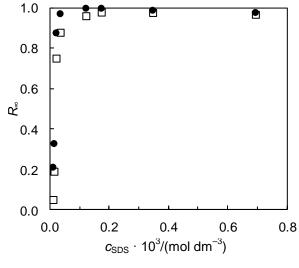
Fig. 6. Influence of SDS concentration on the Al ( $\bullet$ ) and Cu ( $\square$ ) final removal ratio:  $c_{0\text{Al}} = c_{0\text{Cu}} = 1.5 \times 10^{-4} \text{ mol dm}^{-3}$ ,  $u_{\text{G}} = 1.51 \times 10^{-3} \text{ m s}^{-1}$ , pH = 8.0.
