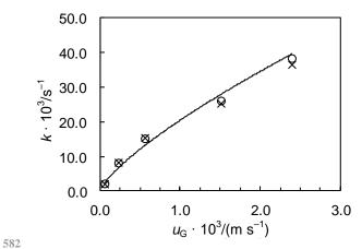
Fig. 8. Influence of the air flow rate on the Al ( $\circ$ ) and Cu ( $\times$ ) flotation rate constant during the foam separation:  $c_{0\text{Al}} = c_{0\text{Cu}} = 1.5 \times 10^{-4} \text{ mol dm}^{-3}$ ,  $c_{\text{SDS}} = 0.94 \times 10^{-3} \text{ mol dm}^{-3}$ , pH = 8.0.
