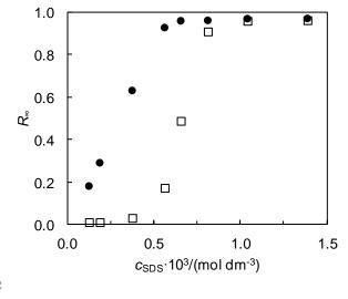
**Fig. 4.** Influence of SDS concentration on the Al (•) and Cu (□) final removal ratio:  $c_{0\text{Al}} = 564$   $c_{0\text{Cu}} = 1.5 \times 10^{-4} \text{ mol dm}^{-3}$ ,  $u_{\text{G}} = 1.51 \times 10^{-3} \text{ m s}^{-1}$ , pH = 3.0.
