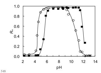
Fig. 2. Influence of the initial pH on the Al ( $\circ$ ,  $\times$ ) and Cu ( $\blacksquare$ , +) final removal ratio using SDS ( $\circ$ ,  $\blacksquare$ ) and CTAB ( $\times$ , +).  $c_{0\text{Al}} = c_{0\text{Cu}} = 2 \times 10^{-3} \text{ mol dm}^{-3}$ ,  $c_{\text{SDS}} = 1.56 \times 10^{-4} \text{ mol dm}^{-3}$ ,  $c_{\text{CTAB}} = 1.65 \times 10^{-4} \text{ mol dm}^{-3}$ ,  $u_{\text{G}} = 1.51 \times 10^{-3} \text{ m s}^{-1}$ .
