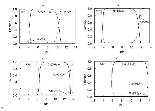
**Fig. 3.** Dependencies of the Al(III) (a, b) and Cu(II) (c, d) forms on the pH value of the aqueous solution (Puigdomenech, 2010). The relations are valid for simultaneous presence of Al and Cu in an aqueous solution. Other than the shown forms of Al(III) and Cu(II) are not presented because of their negligible concentration:  $c_{0\text{Al}} = c_{0\text{Cu}} = 1.5 \times 10^{-4} \text{ mol dm}^{-3}$  (a, c) and  $c_{0\text{Al}} = c_{0\text{Cu}} = 2 \times 10^{-3} \text{ mol dm}^{-3}$  (b, d).
