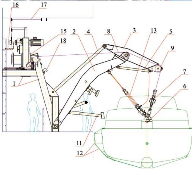
**Fig. 2.** The life boat quadrant davits. Up – a photo of the davits in voyage position; down - in the position along ship side for embarking the people on the lifeboats from evacuation deck
