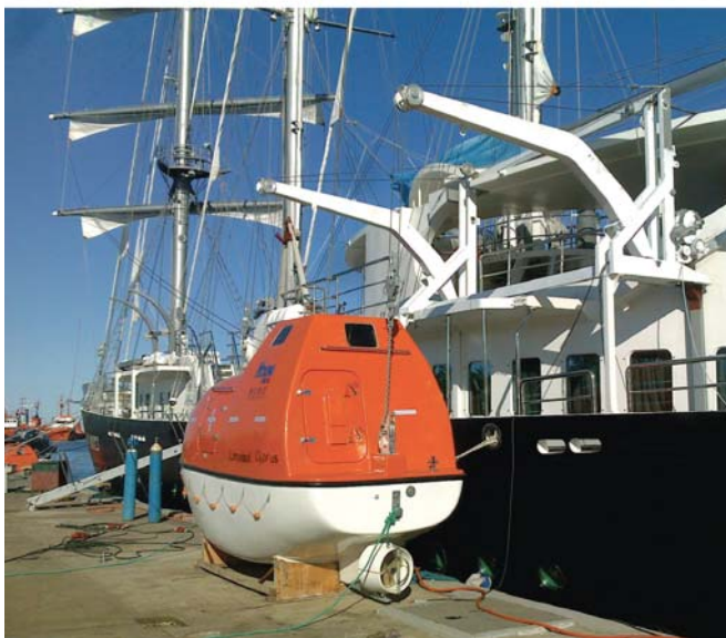
Fig. 4. The life boat davits during and after installation of them on a sailing passenger ship.
