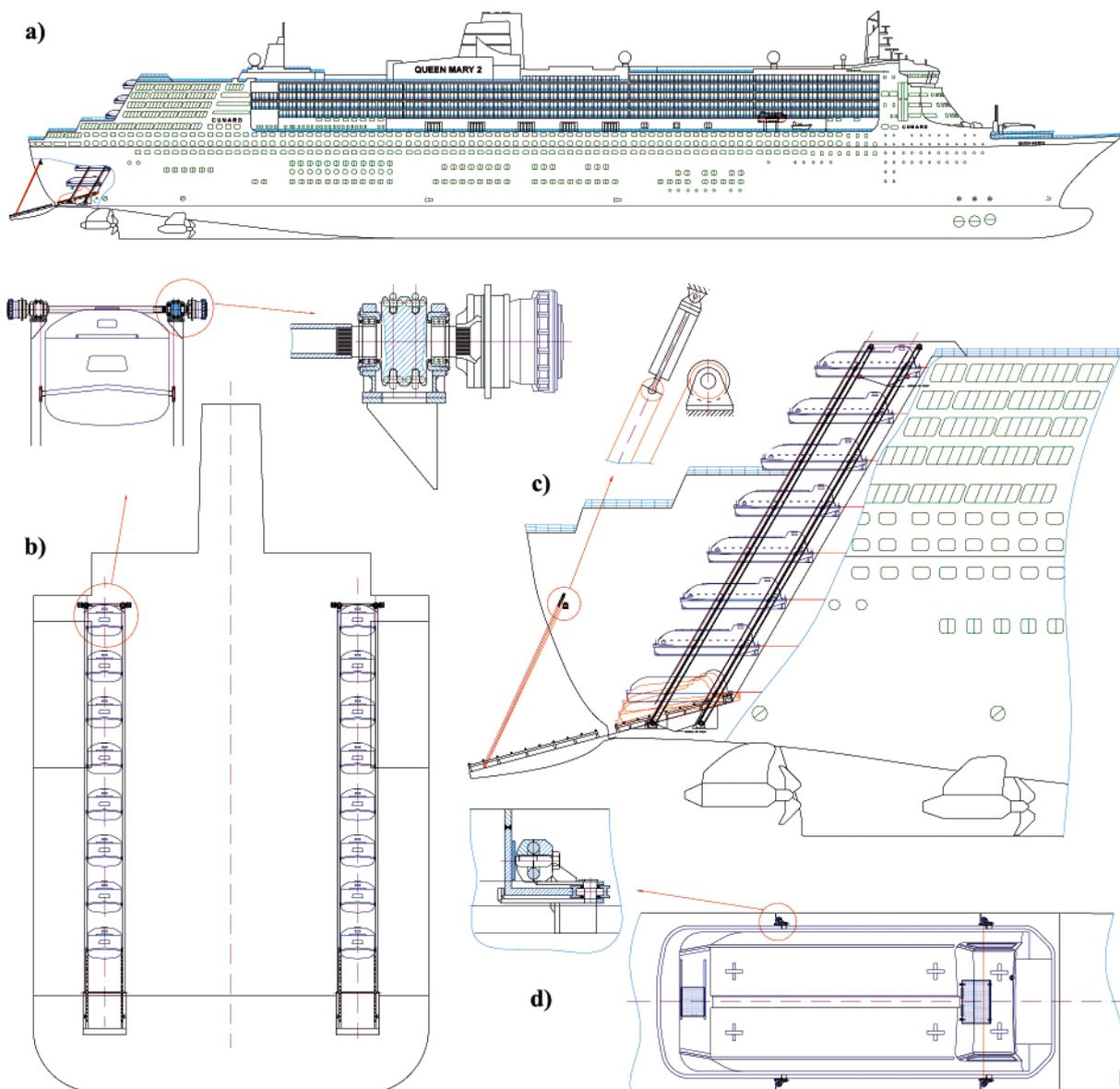
**Fig. 6.** General concept of the device for evacuating the people: **a)** Side view of the ship with the installed device; **b)** rear view of the ship with visible elements of the drive system; **c)** cross-section of the casing with chain lifts and boats and visible mechanism for opening the port-ramp; **d)** top view of the boat placed on the lift in the casing, with visible elements of seating of the boat on the lift.
