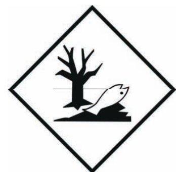
17. Sign for environmentally hazardous material Source: [16]
