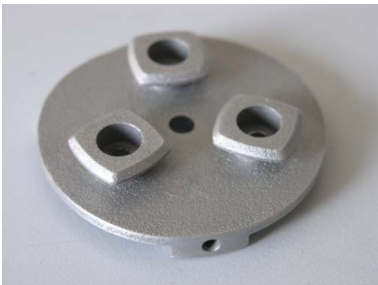
Fig. 7. Stator – contra-mass of the multicell piezoelectric motor
