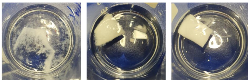
Figure 5. Porous matrices after immersion in PBS solution: PLA/PVA after 5 min (left), PLA/PVA-SiO 2 (middle) after 1 h, and PLA/PVA-CH (right) after 1 h.
