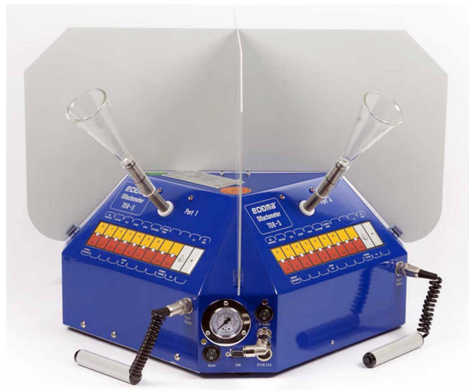
Figure 4. Example of a dynamic olfactometer
