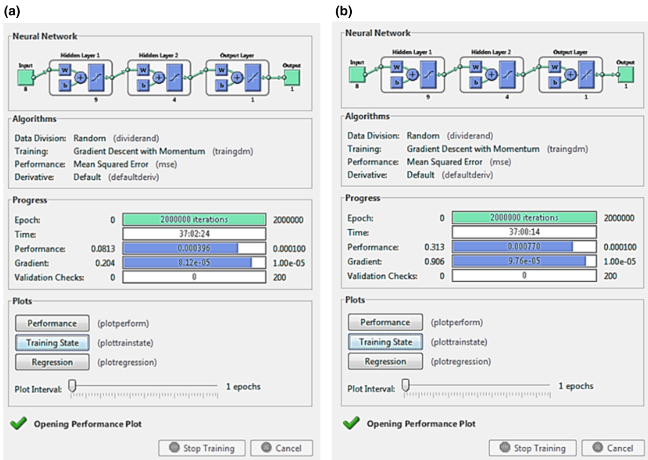
Fig. 6 MATLAB diagrams of pattern recognition networks for ANN model outputs for: a hourly fuel consumption rate; b instantaneous speed over the ground
