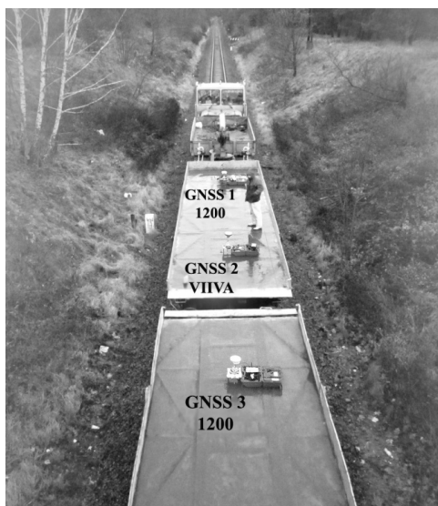
Rys 1. Platforma pomiarowa z zamontowanymi odbiornikami GNSS w trakcie objazdu trasy Fig. 1. Measurement platform with GNSS receivers during the round on surveyed section
