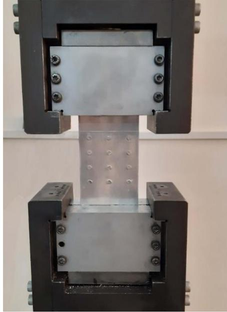
Fig. 3. Experimental test setup for fatigue life estimation.
