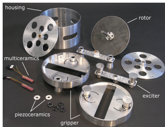
Fig. 12. Disassembled prototype hybrid piezoelectric motor [6]
