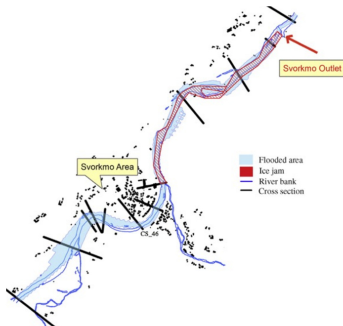
Figure 3. Ice jam on the Svorkmo River affecting the operation of a downstream hydro-power generation facility (from [12]).
