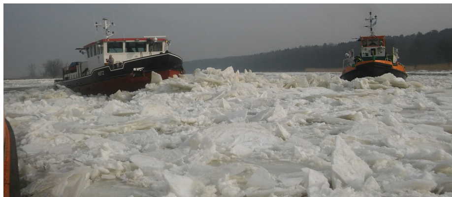
Figure 10. Icebreakers releasing an ice jam on the Oder River (source: RZGW, Szczecin).
