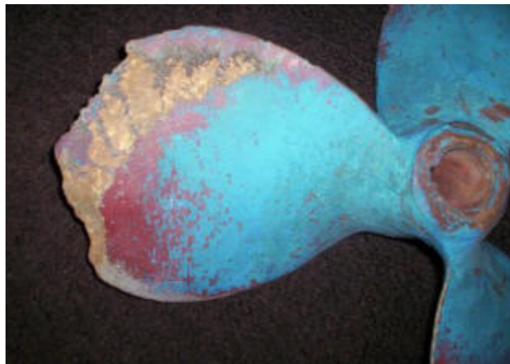
Fig. 1. Cavitation erosion damage of the ship propeller [4]
