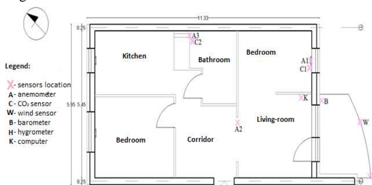
Fig. 3. Floor plan with the location of the sensors
