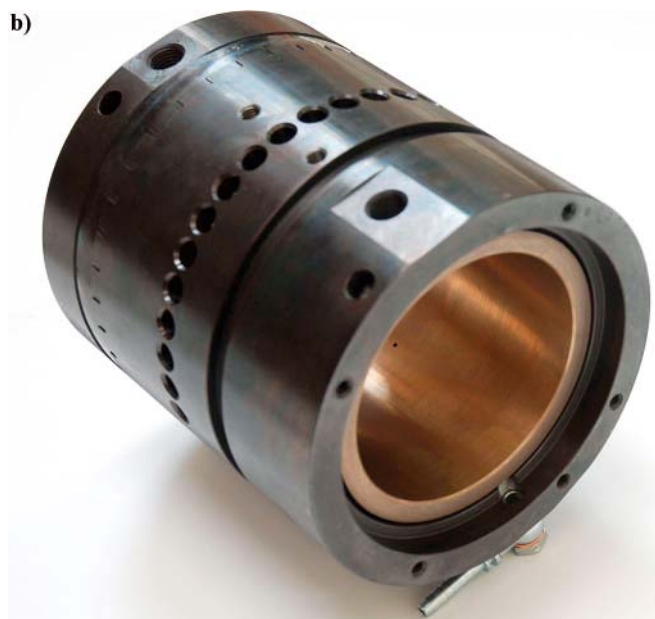
Fig. 2. The tested bearing fitted with metal bush: a) the prefabricated sliding bush element made of sintered bronze, b) the complete bearing before its mounting at the test stand, in which the sliding bush and outer steel sleeve with circumferentially placed sockets for pressure transducers, are seen.
