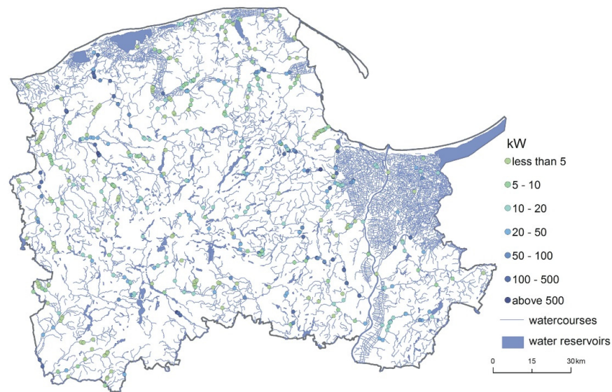
Figure 16. Localization of water dams and power of the potential hydropower plants in the Pomorskie voivodeship (own elaboration).
