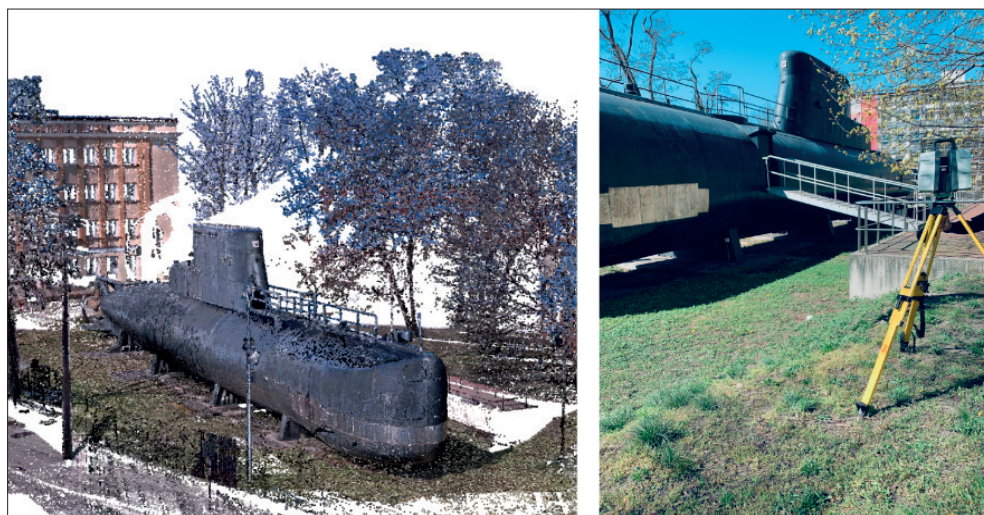
Fig. 1. Point cloud for a Kobben-class submarine (left panel) as measured by a Leica ScanStation P50 laser scanner (right panel)
