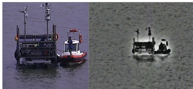
Fig. 12. Image from long-range cameras during the day: visible light camera (left), thermal imaging camera (right)
