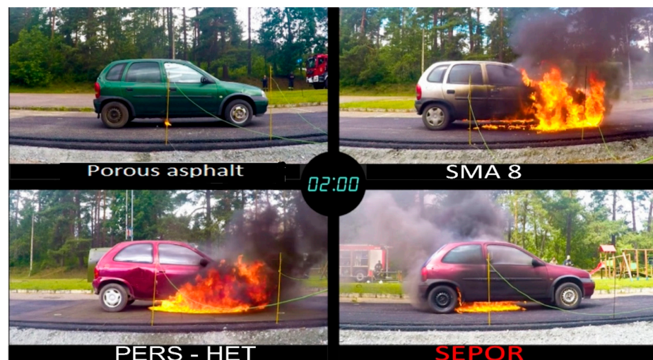
Figure 35. Fire development 120 s after ignition.
