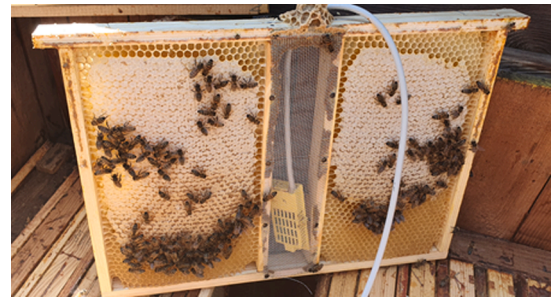
Fig. 2. Hive frame with installed probe.
