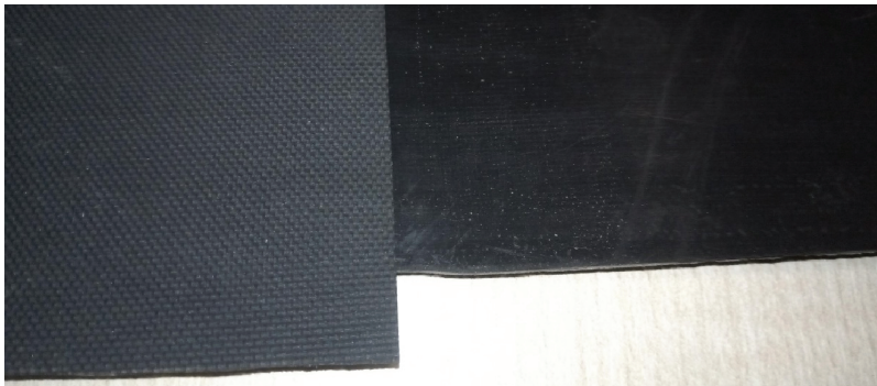
Fig. 2. Two types (outside and inside) EPDM membranes – visible different surface textures on the backside
