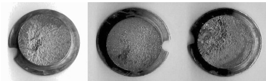
Fig. 9. Surface of the SUPERSTON alloy after cavitation test by 5.25h: a) 4000W, 0.5m/min; b) 4000W, 1.0m/min; c) base material - as casting
