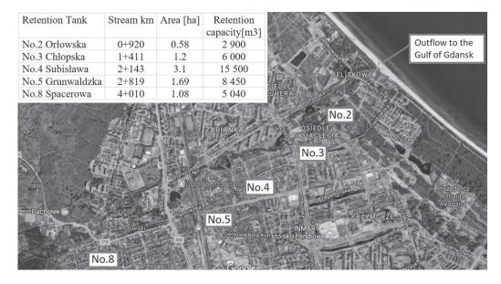
Fig. 1. Locations and retention capacities of analyzed retention tanks on Oliwa Stream.
