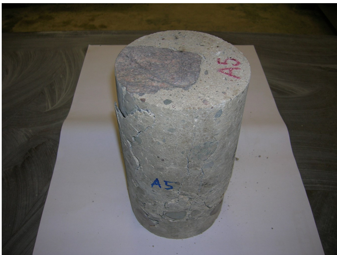
Figure 8. Damaged concrete cores with visible coarse aggregate (stone)
