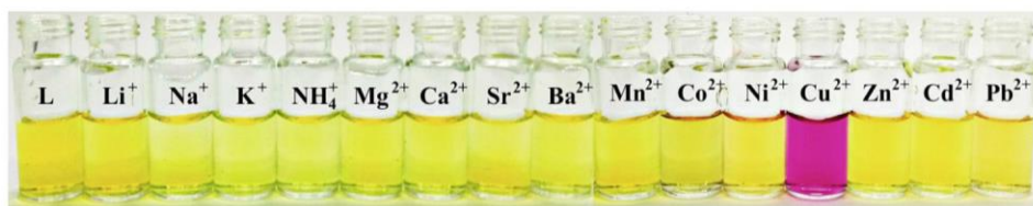
Fig. 13. Color change of ligand ( c_L = 2.16 \times 10^{-5} M) in water-DMSO solution (9:1, v/v) in the presence of ammonium and metal chlorides (pH 6.0).
