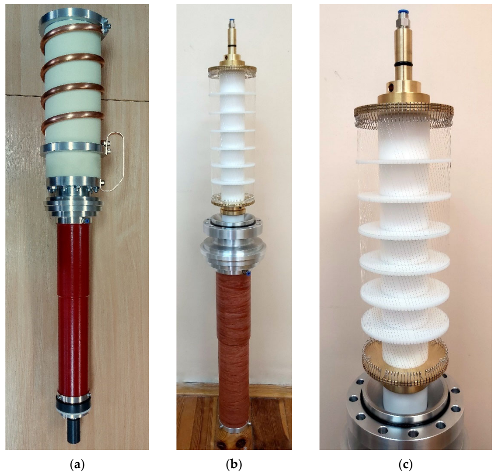
Figure 13. Photographs of the integrated and compact high-power pulse generation and forming system (a), along with a view of the inside of the forming fuse compartment (b,c).
