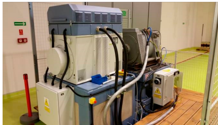
Figure 5. Measurement setup with the dynamometer (on the left) and the studied synchronous generator (on the right).
