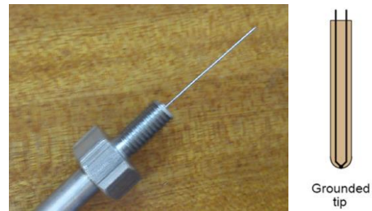
Fig. 2. Photo and cross-section of a type K thermocouple used in rapidly variable measurements
