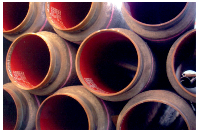
Fig. 1. Thick-walled steel pipe coated with 3M Scotchkote epoxy coating EP2306 HF, and a heavy concrete coating, for 370 km × 48 in. Dolphin (subsea) gas pipeline [10]
