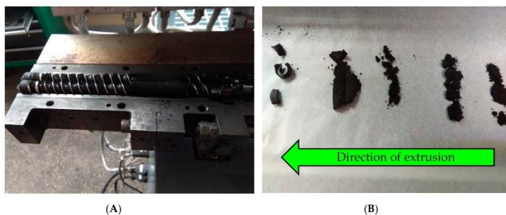
Figure 5. The appearance of: (A) open extruder barrel after stopping of reclaiming process (B) GTR collected from different zones of the extruder barrel.
