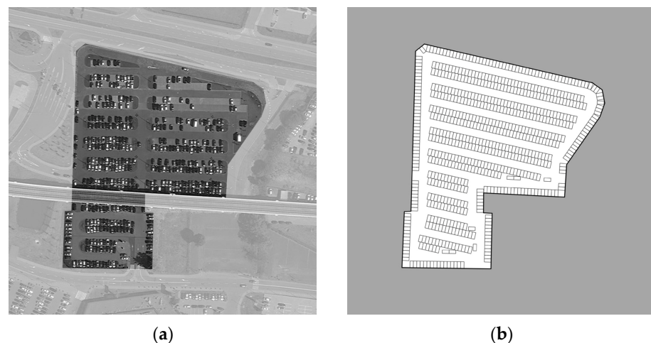
Figure 7. Comparison of parking layouts, location: Juliusza Słowackiego 200, Gdańsk, Poland: (a) Existing solution with 537 parking spots; (b) Best solution generated by the algorithm with 690 parking spots (153 more spots or 1988.30 square meters of green area). Input parameters—street width: 600 cm, spot width: 250 cm, spot length: 500 cm.
