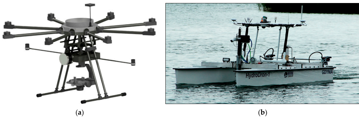
Figure 6. Aurelia X8 UAV with the mounted prototype optoelectronic module (a) and the “HydroDron” USV (b).
