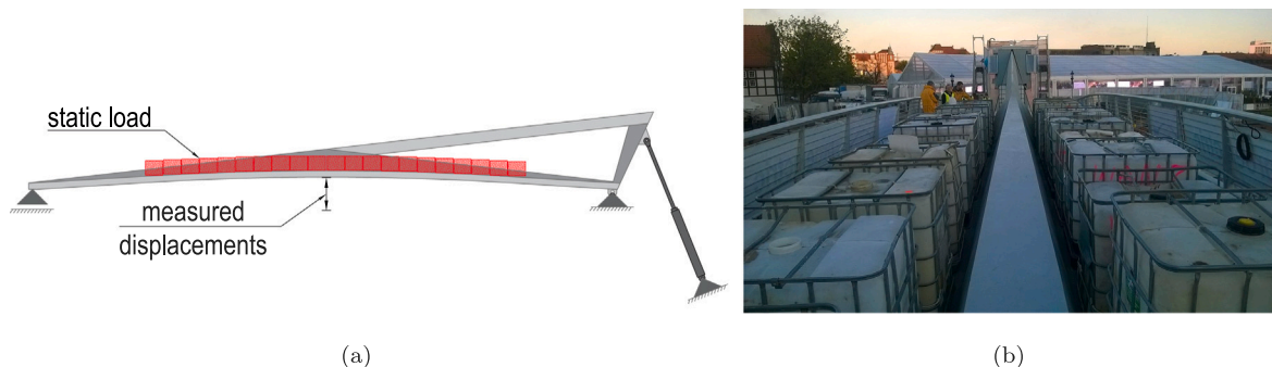
Fig. 19. The static load during the field test: (a) side view with the measurement point marked; (b) the water tanks during the field test.
