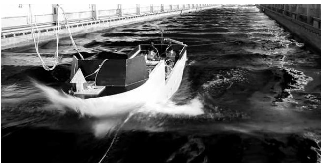
Fig. 1. The model of a ship in towing tank while seakeeping test
